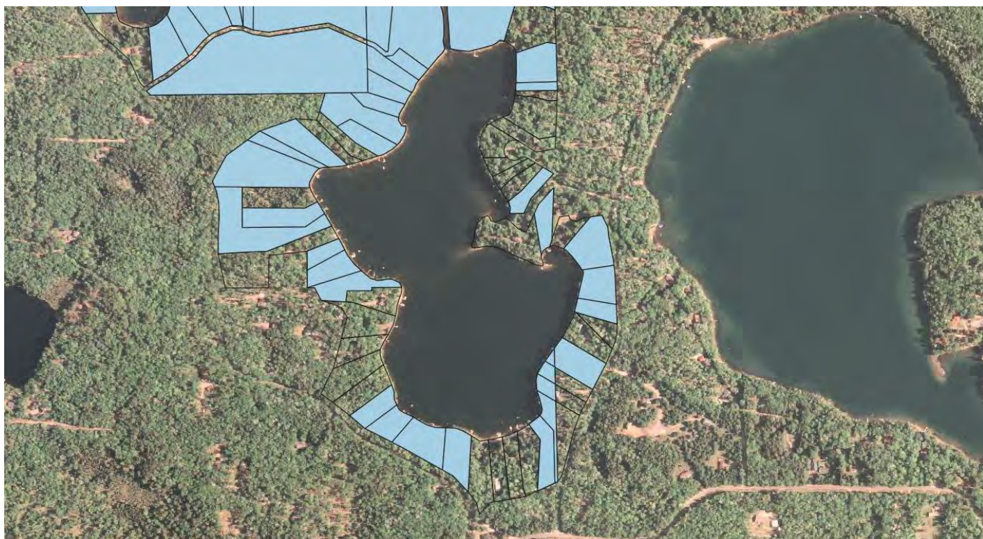
Figure 4. Alma Lake tax parcels shaded in blue have shoreland with greater than 60% of the buffer area in native trees, shrubs, forbs, and grasses.
